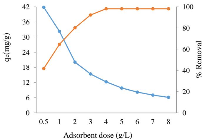
Fig. 4. Effect of adsorbent mass on adsorption of 50 mg /L CIP onto ARM
