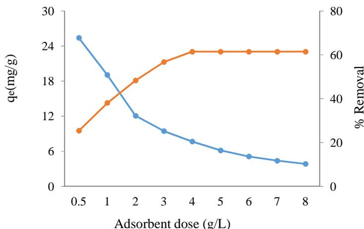
Fig. 3. Effect of adsorbent mass on adsorption of 50 mg /L CIP onto RM
